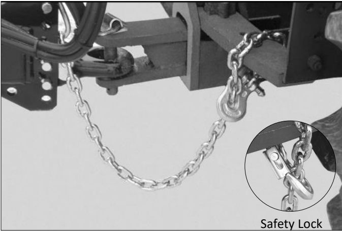
Figure 3 Install safety chain to tractor hitch. Be sure safety lock is in the magnified position.
